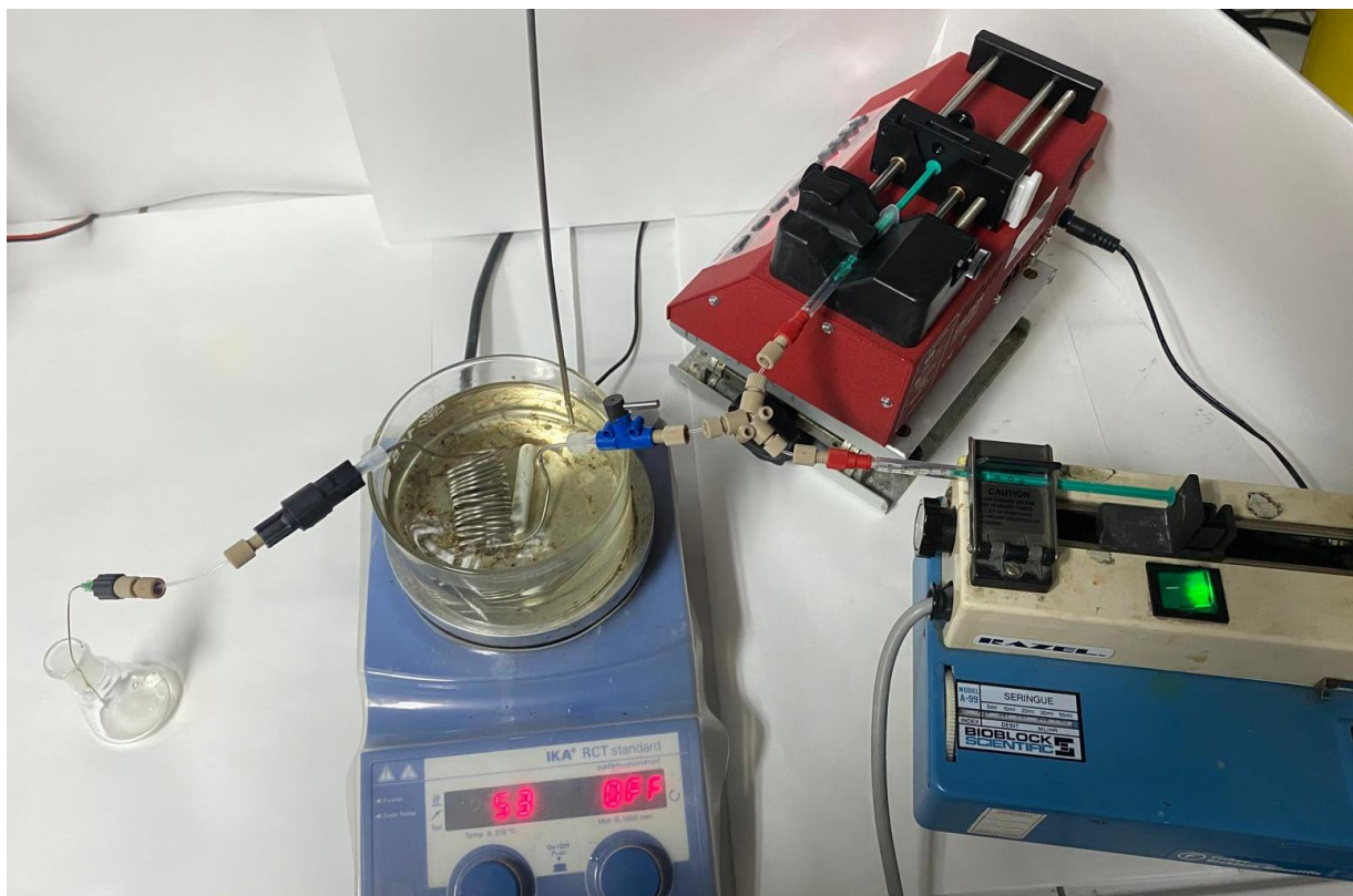
Figure S4 Details of the setup used for the thermal step in flow.
