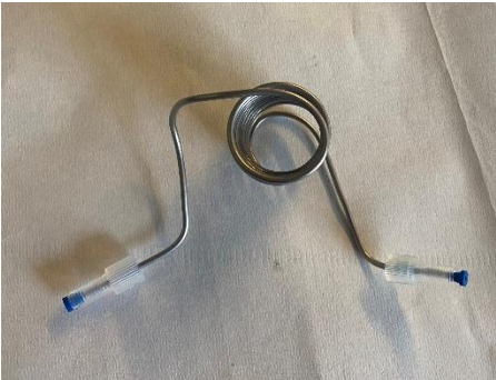
1 mL Coil Tubing, Stainless Steel 1/8" OD x 1 mm ID
