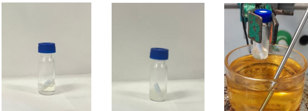
Figure S1 Details of the condensation reaction in batch of a and a' (1 mmol scale). Left: t = 0 min; T = 25 °C; Center: t = 1 min; T = 25 °C; Right: t = 100 min; T = 50 °C.
