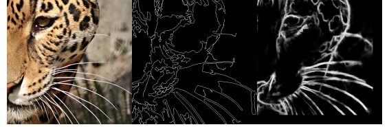
Fig. 2 The figure presents a comparative visualization of edge detection results from the same input image (left). The middle image shows the output of the Canny detector[2]. The right image displays results from the HED detector[3].
