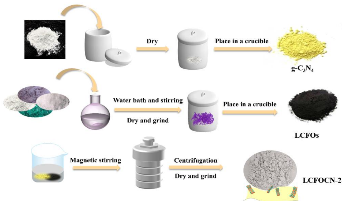
Figure S3 Synthesis processes of a series of LCFOCNs photocatalysts.
