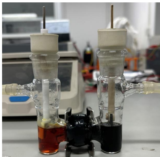
Figure S2. Reaction set-up of divided cell
