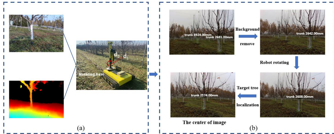
Fig. 4 The schematic diagram of target trunk detection and localization. (a) Image acquisition and model application. (b) Target trunk acquisition. The numbers in the image represent the detection distance of the trunk
