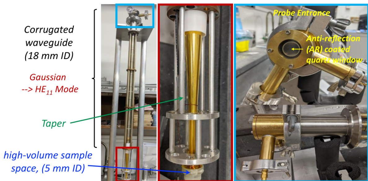
Supplementary Figure 5: Detail of the 1.16 m long cryoprobe showing radiation baffles, anti-reflection coated quartz window, 18 mm to 5 mm ID taper and 50 mm long 5 mm ID sample section.
