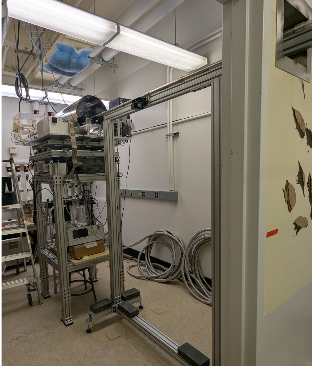
Supplementary Figure 8: The spectrometer's transmitter assembly including the TWT tube and its high voltage modulator and modulator control box, mu-metal magnetic shield and helically corrugated waveguide, 12 ft.
