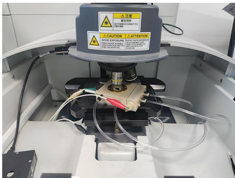
Supplementary Fig. 21 | The electrochemical cell for Operando Raman measurements. A water immersion objective and a 532 nm laser were used. An Ag/AgCl (saturated KCl) electrode and a Pt wire were used as the reference and counter electrodes, respectively.
