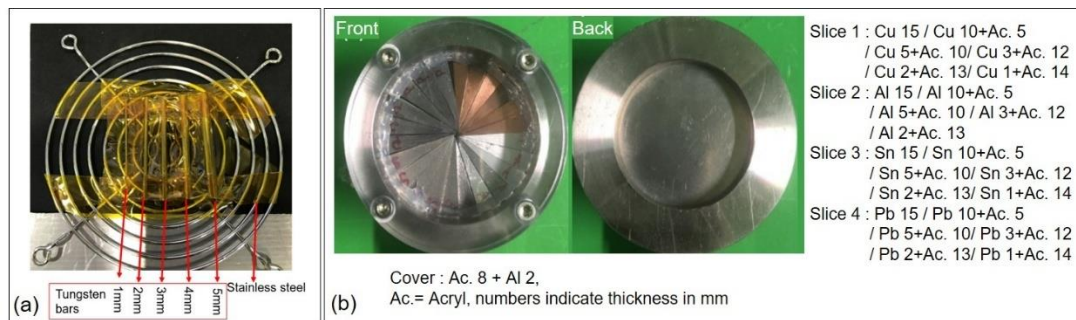
Fig. S2| (a) A metallic structure, consisting of tungsten bars of varying thicknesses and stainless steel rings, was used for radiography and (b) an attenuation filter composed of different materials and thicknesses
