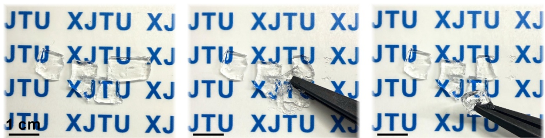
Supplementary Figure 29. Demonstration of weak mechanical properties of PNIPAM hydrogels.
