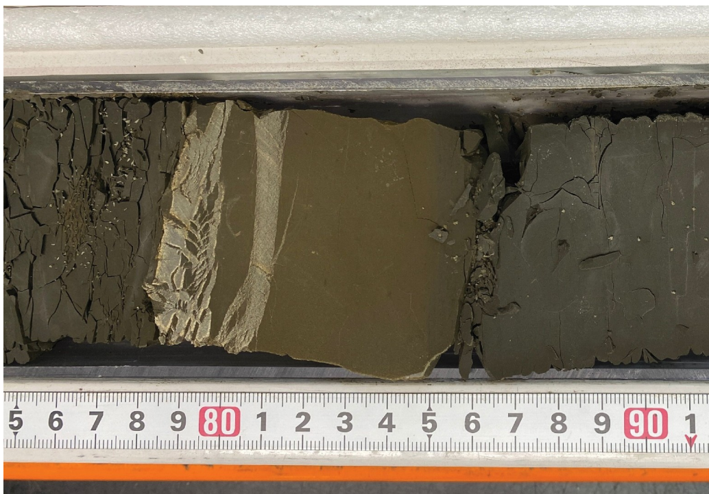
Figure 5: Core photograph of sample 72R-3A-75/100. Zebra-like textures formed by light calcite veins within the brown siderite-rich claystone (core distance of 78-82 cm).
