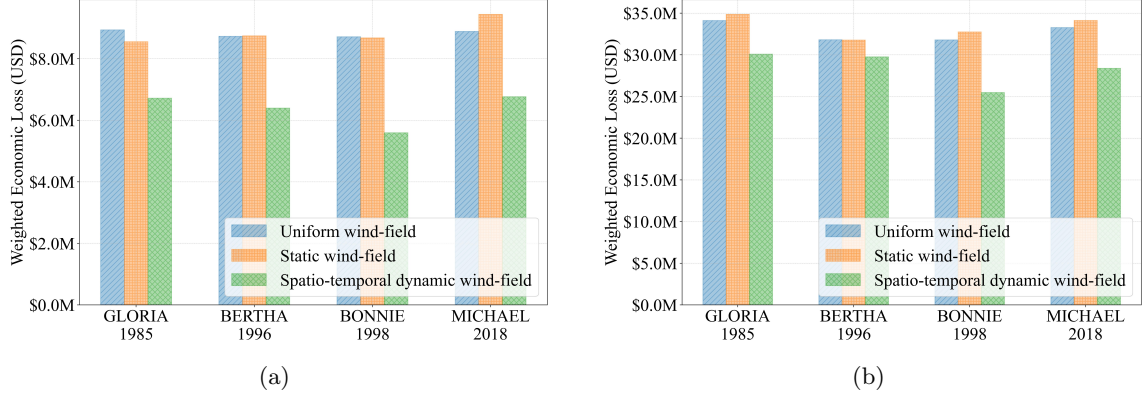
Supplementary Figure 15: Weighted economic losses after resilience optimization under different wind-field modeling approaches for (a), Suffolk City and (b), Chesapeake City. Bar charts demonstrate that high-spatio-temporal-resolution (HSTR) dynamic wind field modeling consistently reduces economic losses compared to uniform and static peak wind models across all hurricane approach directions, providing quantitative validation of the economic benefits achievable through enhanced meteorological data integration in urban power distribution networks planning.
