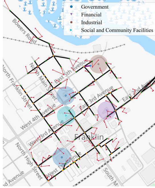
Supplementary Figure 4: Critical infrastructure identification through automated geospatial mapping methodology. Example demonstration of the proximity-based building classification process in Franklin, Virginia, showing how electrical load nodes are systematically matched to OpenStreetMap building types based on distance optimization and geometric constraints, enabling accurate identification of hurricane-vulnerable critical facilities for prioritized resilience planning.
