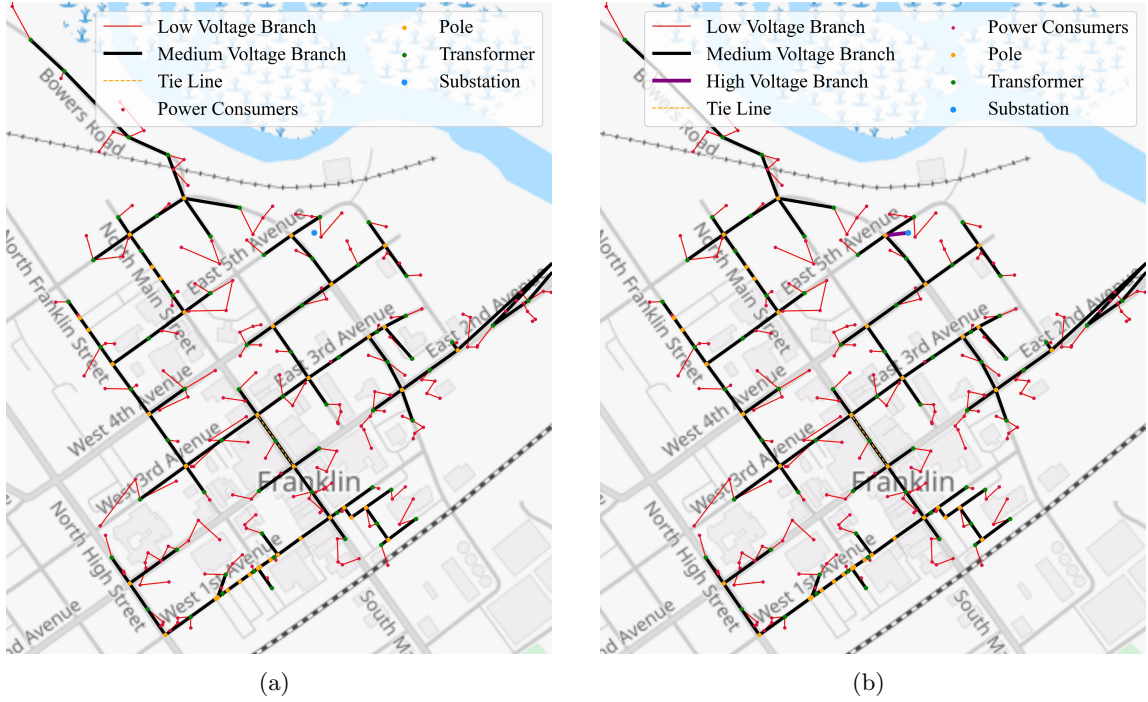
Supplementary Figure 2: Hierarchical synthesis of medium and high voltage distribution infrastructure for climate resilience analysis. (a) Optimized medium voltage distribution network showing radial feeder configuration connecting low-voltage transformers to substations through strategic pole placement and routing optimization. (b) Integrated high voltage distribution network providing bulk power delivery by distribution substations across the regional service territory, forming the backbone infrastructure for urban electricity supply.
