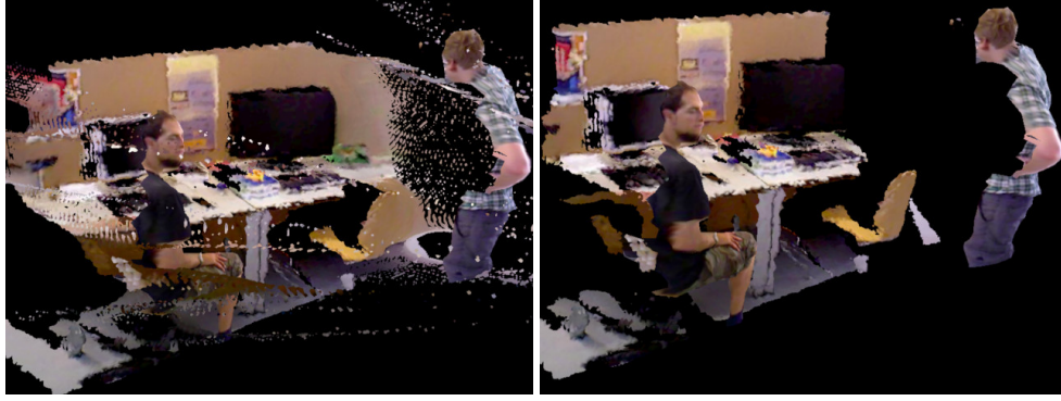
Fig. 4: Comparison of Mono2VR run on the ‘walking xyz’ sequence using ground truth depth data with inpainting (left) and without inpainting (right). Inpainting on TUM sequences creates floaters around object boundaries—note the areas around the two people in the scene and the gray colored floaters.
