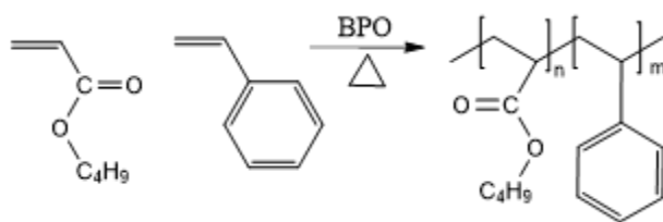
Figure 1. St-co-BuA (83:17) reaction scheme
