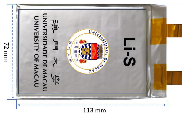
Supplementary Fig. 38 | Dimensions (length and width) of the pouch cell.
