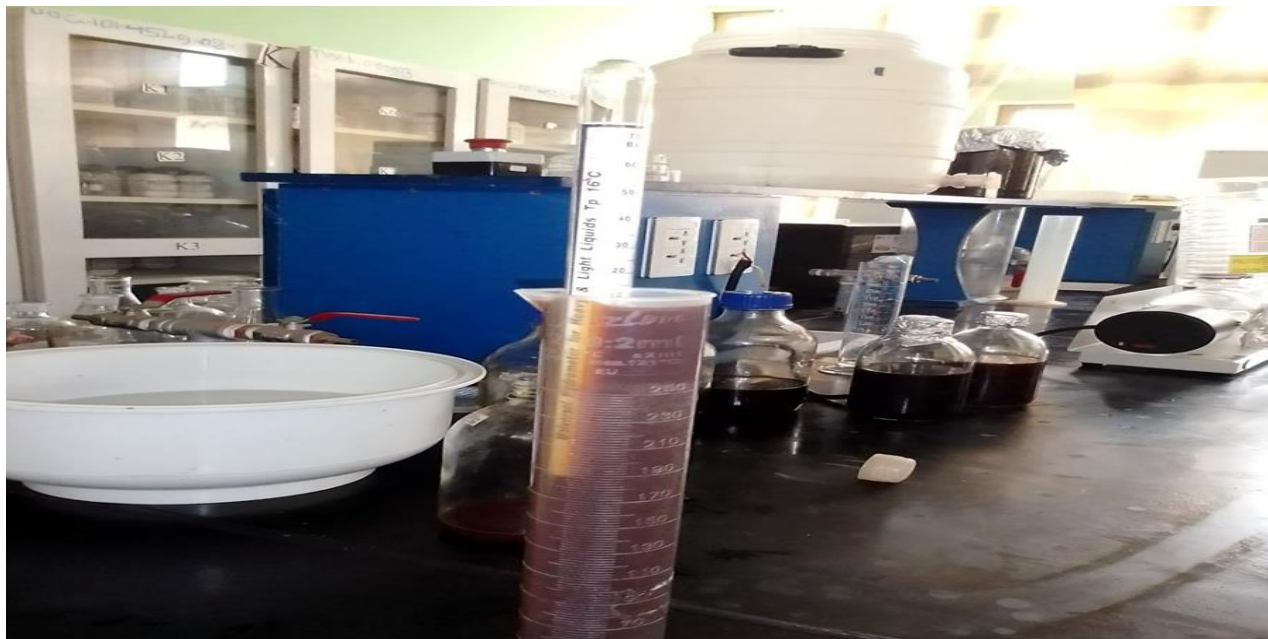
Figure S3: Specific gravity of sugar beet juice measured with a Baume hydrometer.
