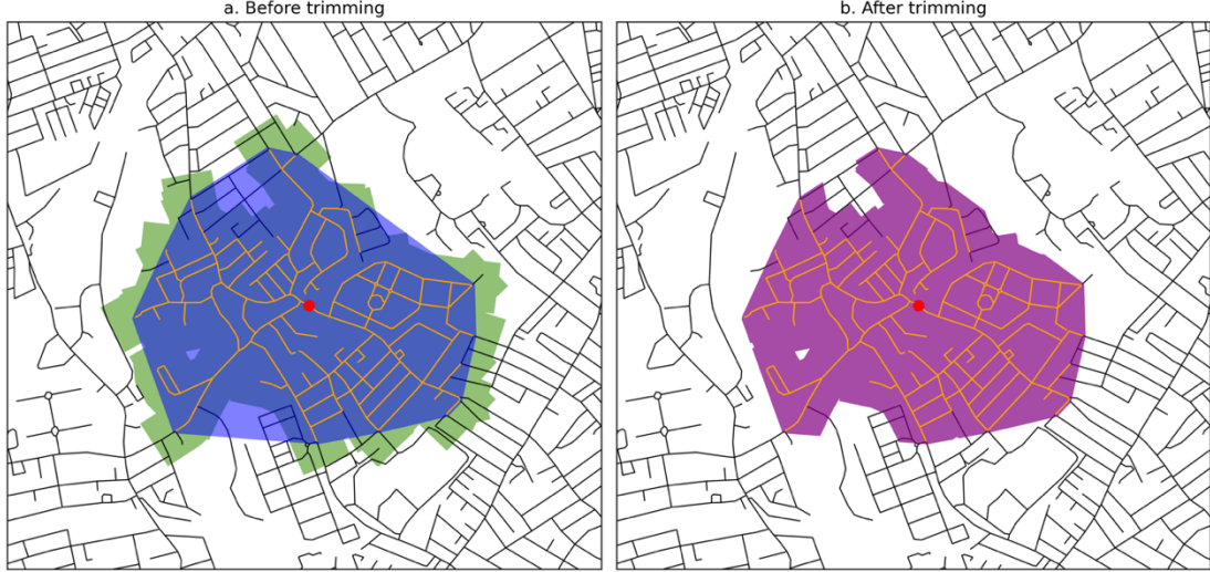
Figure S1-2. Illustrative example of service area construction. Panel (a) indicate the shape of the service area of a particular count point (red point) before trimming (blue polygon). The trimming process involves generating and merging a 100-meter buffer (green polygon) around all traversable roads (yellow lines). Panel (b) shows the resulting service area after trimming (purple polygon), which is the intersection of the blue and green polygons in Panel (a).
