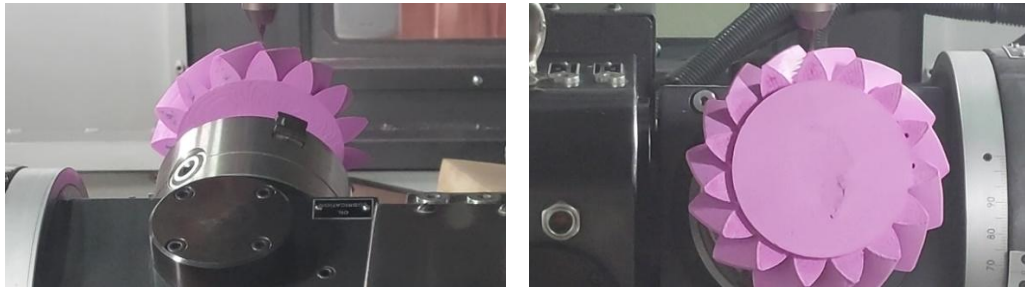
Fig. 7. Spiral bevel gear clamped on a 5-axis machining centre.
