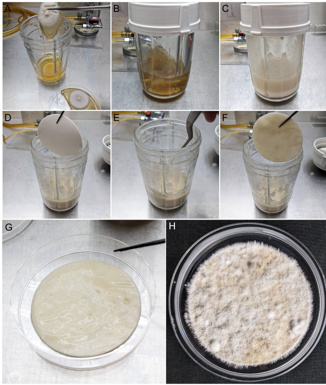
Figure S2: First-stage procedure. (A, B) Colonies in blender; (C) mycelial suspension; (D–G) dipping filter papers; (H) colonized filter paper after 5 days.
