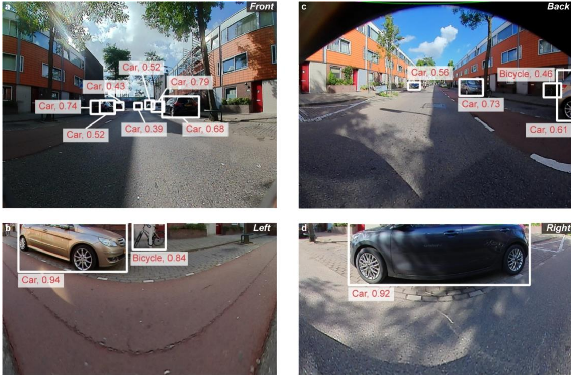
Figure S22. Object recognition after the large-scale tensor processing using our CNT analog tensor core. The object recognition results in the (a) front, (b) left, (c) back, and (d) right view of the street after the distortion correction and edge detection tensor processing. The cars and bicycles are accurately recognized with high confidence, proving the effectiveness of performing tensor processing using our analog tensor core.
