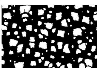
Figure S32. Image analysis of different concentrations of middle-reflector to quantify the SiO x -np uncovered areas. Filling height ( h ) is calculated from the percentage of uncovered areas. The height of the pyramid tip ( H ) is taken as 260 nm.
