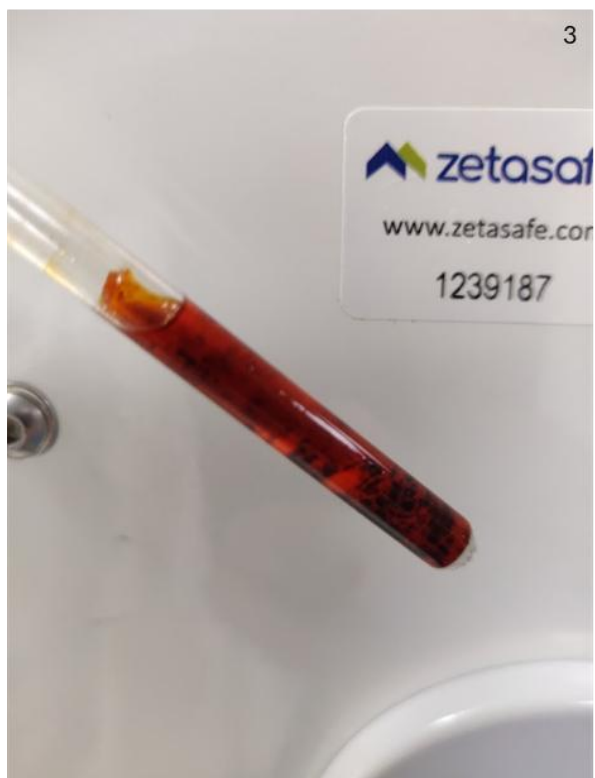
Figure S 23: Colour progression of the reaction of 2^{m-xyI} immediately subsequent to the addition of 1 bar of ethylene gas to afford 9^{m-xyI} .
