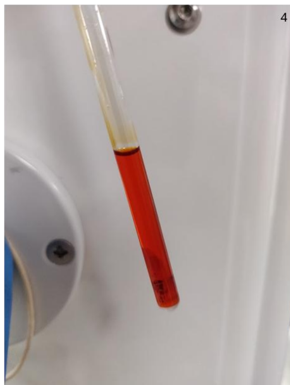
Figure S 23: Colour progression of the reaction of 2^{m-xyI} immediately subsequent to the addition of 1 bar of ethylene gas to afford 9^{m-xyI} .
