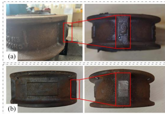
Fig.28 Comparison of physical model before and after grinding: (a) before grinding;(b) after grinding
