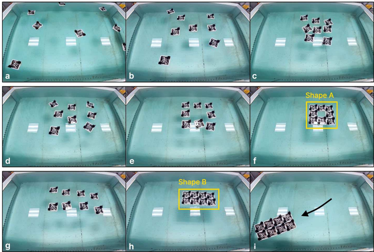
215 Fig. 3. Self-reconfiguration experiments with eight FloatForm modules. (a) Idle robots awaiting a target 216 shape command. (b)-(c) The robots begin gathering within the approximate boundary of a target shape, 217 “A”. (d)-(e) Once the boats are within the boundary, discrete positions are assigned to each unit. (f) The 218 boats then latch together to form a rigid structure. (g) A new target shape, “B”, is received: the boats de- 219 latch and the process repeats, as they reposition within the boundaries of shape “B”, where discrete positions 220 are reassigned, and the boats latch into the new configuration (h). (i) The newly formed structure maneuvers 221 to the side of the pool.
