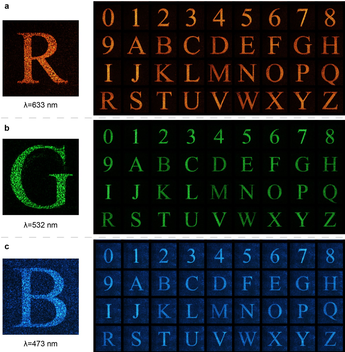
Fig. S23. Experimental demonstration of Fresnel holographic display.
