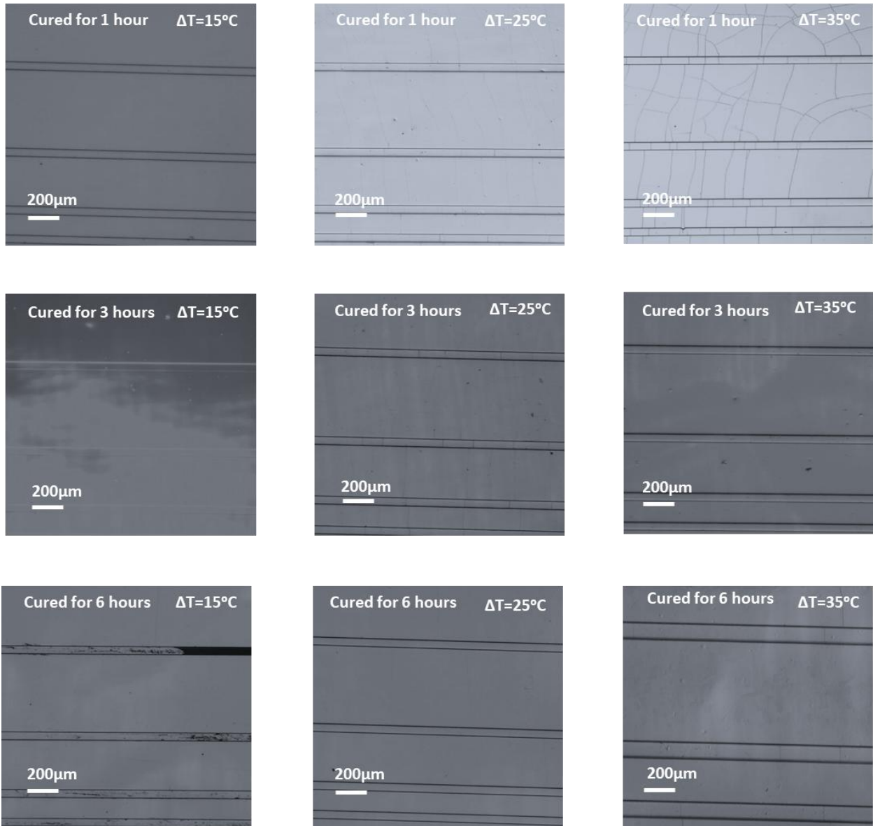
Figure 13 | Optical microscope images illustrating the absence of wrinkles in bilayer systems, consisting of 100nm \text{As}_2\text{Se}_3 thin films deposited on PDMS 5 substrates, when heated to temperatures lower than the optimum temperature range for the bilayer system. The PDMS substrates were cured for 1 hour (Top), 3 hours (Middle), and 6 hours (Bottom). The thermal expansion coefficient being higher in PDMS substrates cured for 1 hour, during heating the tensile stress acting over the film deposited atop is also higher leading to the formation of cracks as seen in the Top Right image. For substrates cured for 3 hours and 6 hours, cracks are absent.
