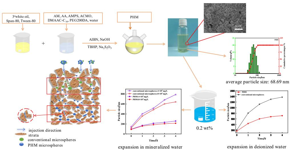
PHM microsphere initial particle size of 68.69nm, in 80°C (deionized water) in the expansion of 4 days, the expansion times for 4.34 times; 25°C (mineralized water) in the expansion of 4 days, the expansion times for 2.34 times, the blocking rate is greater than 85%.
