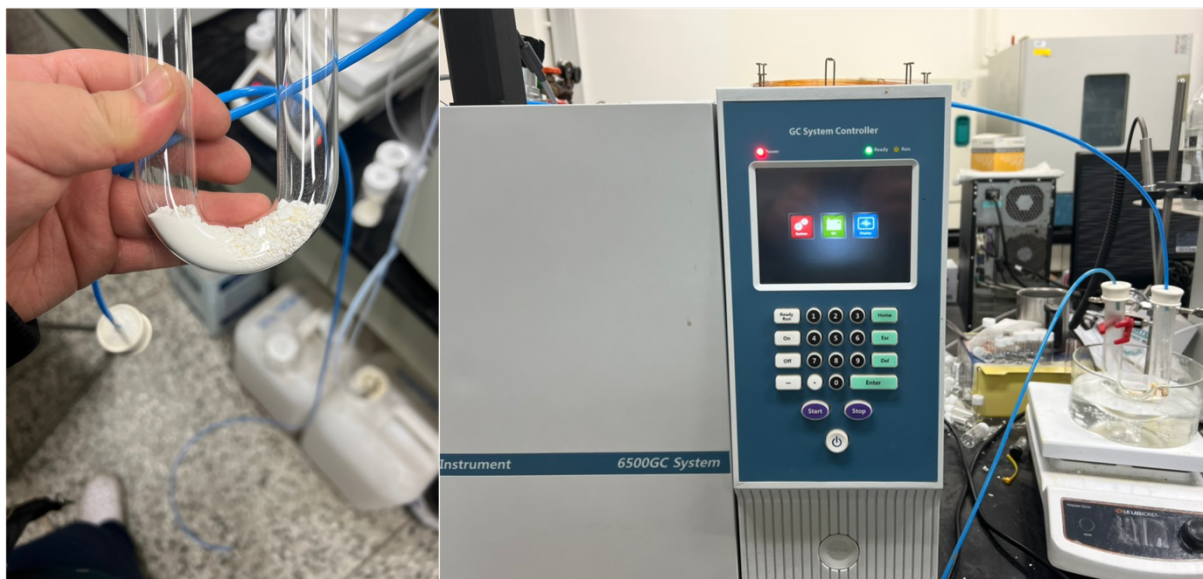
Fig. S27. Photographs of Set-up for breakthrough measurement to analyze selectivity.
