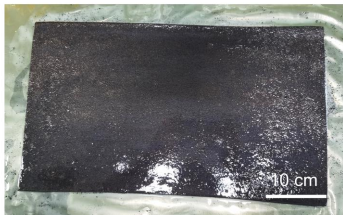
Figure S15. The digital photo of PGC after vacuum infusion. Photo Credit: Kai Pang, Zhejiang University.
