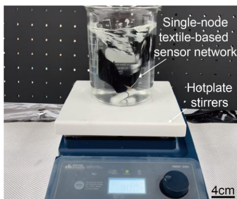
Supplementary Figure 11. Photograph showing the experimental setup for washing stability test of the textile-based sensor network. The washing protocol included sequential stirring steps of 30 minutes in 40°C DI water, 30 minutes in 40°C DI water with detergent, followed by drying step in a forced convection oven for 50°C for 30 minutes.
