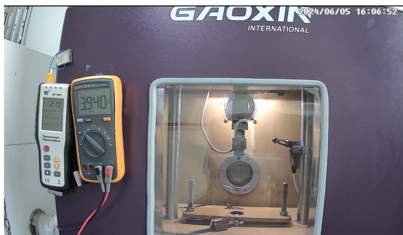
Video S5. Nail penetration test of E3 (EC/DEC-based) with 18650 cylindrical cell.
