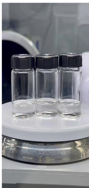
Video S9. Immersion tests of sodium-deposited HC anode. (Left) EC/DEC; (Middle) TMP; (Right) TEP.
