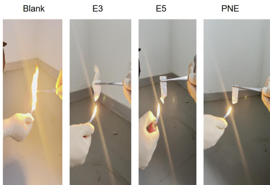
Video S1-S4. Ignition experiment videos of fresh separator (Video S1) and the separators immersed in E3 (Video S2), E5 (Video S3) and PNE (Video S4).
