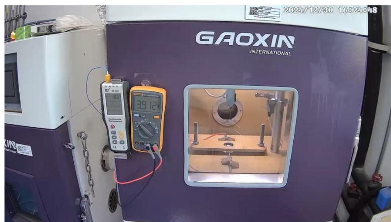
Video S6. Nail penetration test of E5 (TMP-based) with 18650 cylindrical cell.
