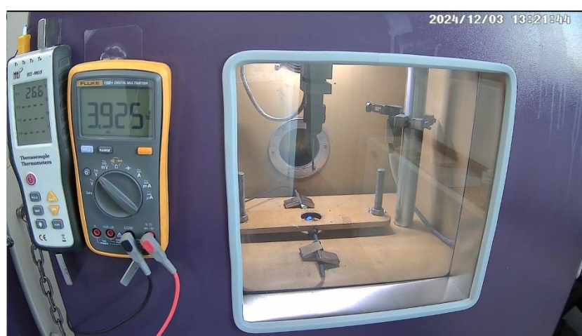
Video S8. Nail penetration test of PNE (TEP-based) with 18650 cylindrical cell.
