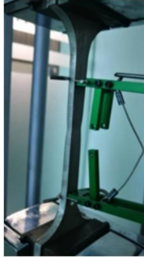
Figure 10. Mounted Specimen with Rupture after the Creep Test
