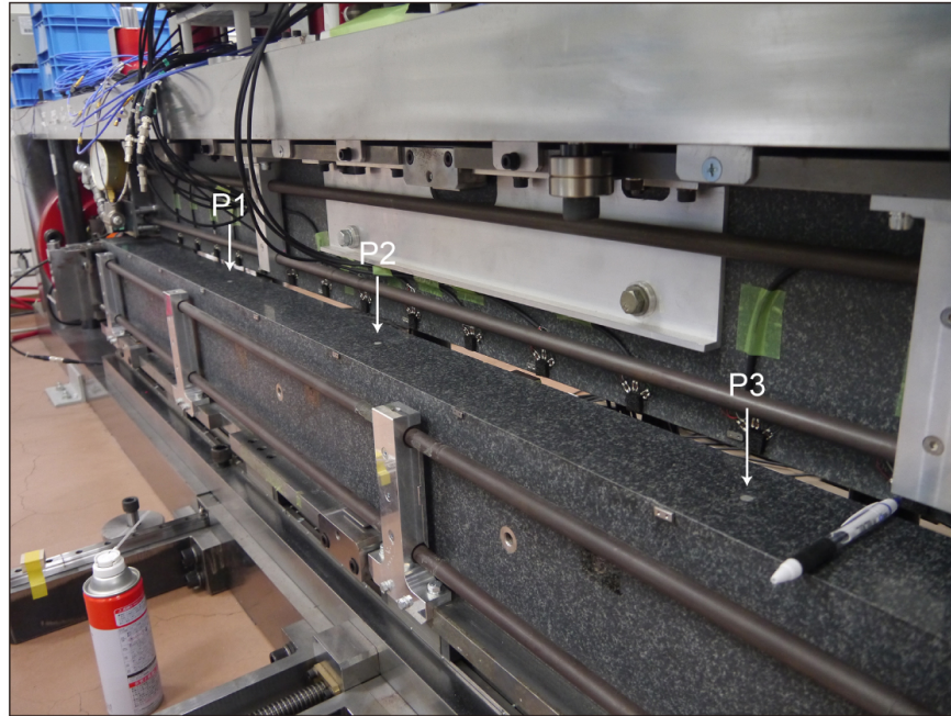
Fig. S2 Photographs of the gouge patch. a , Top view of the GP placed on the fault surface of the bottom rock specimen at patch P3, taken prior to the stick-slip experiment. b , Oblique view of the GPs set on the fault. The bottom rock specimen can be pulled back to facilitate the placement of the GPs. Note that the photograph was taken after the removal of the AE sensors, which had been installed on the side surface of the bottom rock specimen.
