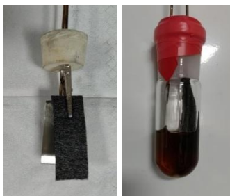
Fig. S32. Electrolysis setup (graphite felt, nickel plate: width 1.8 cm, immersion depth 1.5 cm)
