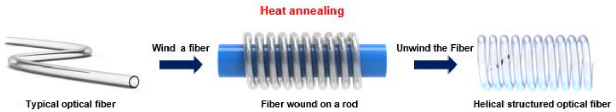
Supplementary Fig 1. Schematics illustration for the fabrication of the 3D helical structure optical fiber sensor.
