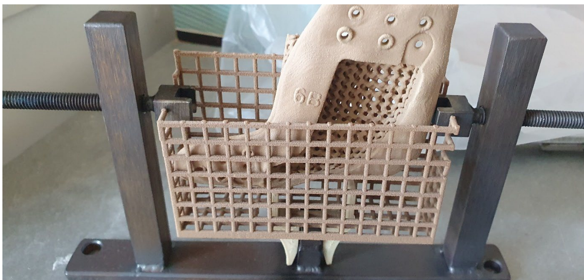
Supplementary Fig. S6: A custom SLS-PEK frame held in the thermal toughening tray.
