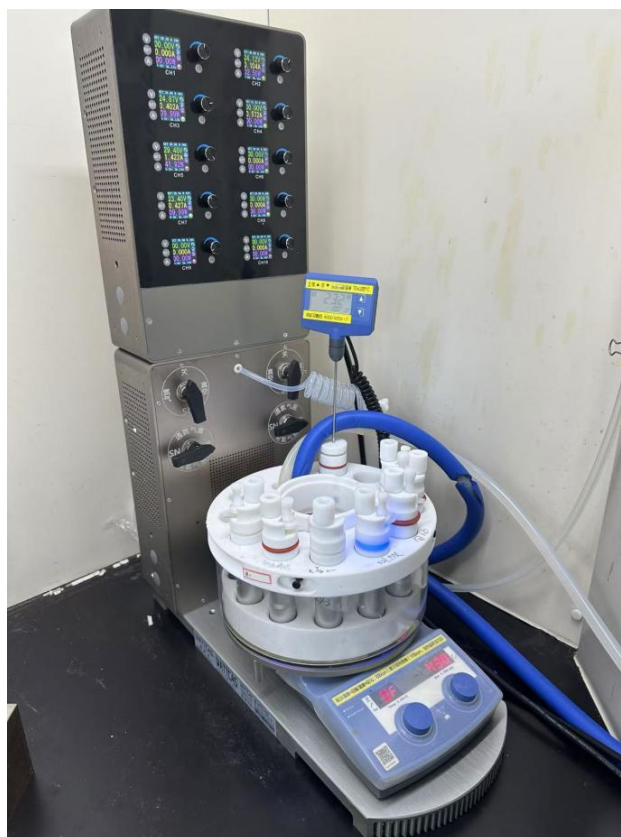
Figure S3. Photograph of the WATTCAS Parallel-Light Reactor (WP-TEc-1020HSL) photoreactor. Reaction was conducted with room-temperature cooling and magnetic stirring in a sealed tube under N 2 atmosphere.
