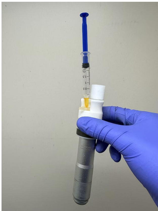
Figure S5. The vessel was under positive pressure, causing spontaneous volume expansion when purged with a needle attached to a 2.0-mL syringe.
