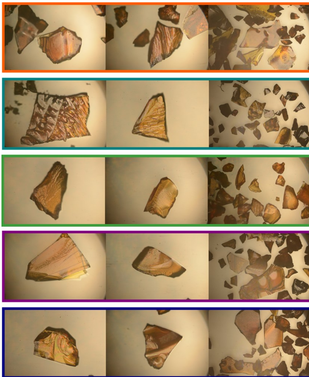
Figure S38. Optical images of different dg-MUV-29-X monolithic glass. Orange corresponds with dg-MUV-29 . Blue corresponds with dg-MUV-29-NH 2 . Green corresponds with dg-MUV-29-CH 3 . Purple corresponds with dg-MUV-29-Br . Dark blue corresponds with dg-MUV-29-Cl . The amount of bim incorporated in all cases corresponds to x = 0.5 .
