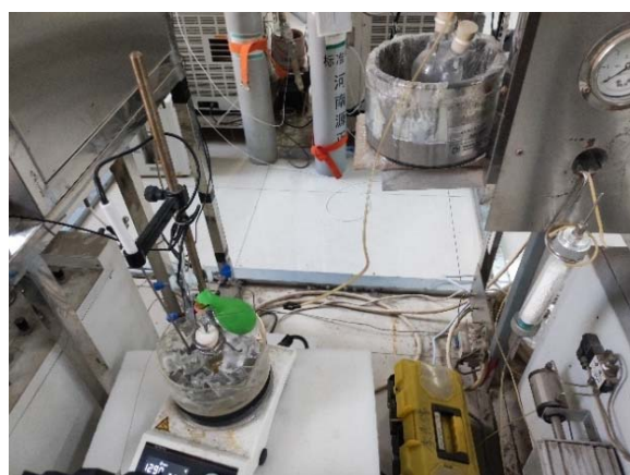
Figure S-18. The device used in oxidative oxidation of propane gas.
