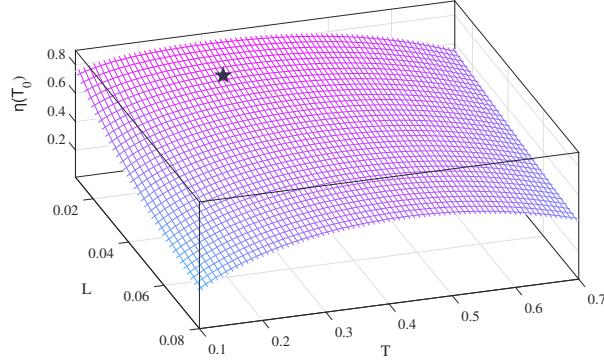
FIG. S1: The dependence of memory efficiency  $\eta(T_0)$  on the transmissivity of the input-output mirror  $T$  and the intracavity loss  $L$ . The black star corresponds the experimentally measured result.
