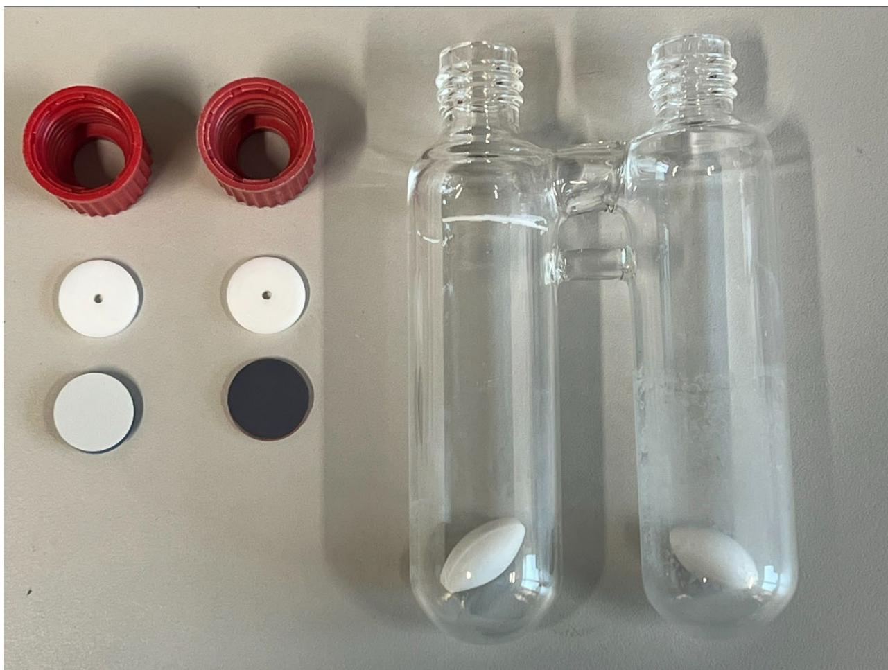
Figure S4. Two-chamber reaction glassware, stir bars, caps, Teflon disks, and silicone seals used for the 250 mg scale hydrocyanation reactions.
