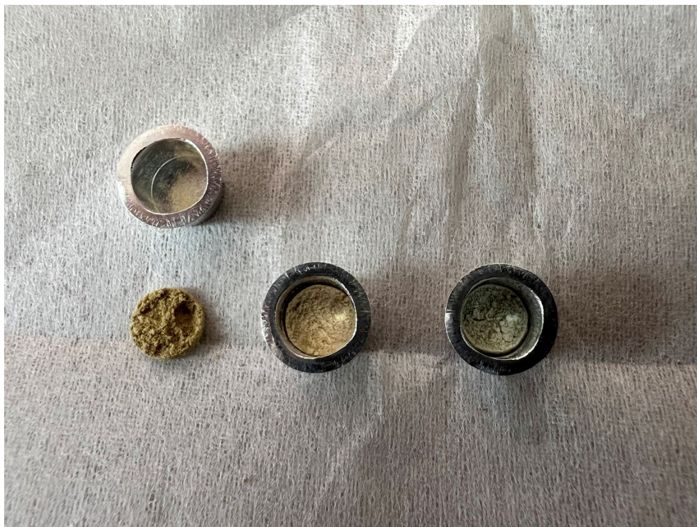
Figure S12. From left to right: H-NBR2-3 , H-ABS2-2 , and H-SAN2-1 after helium for 10 h at 150 °C. Note the agglomerated samples, such as the H-NBR2-3 sample, which was originally a powder.
