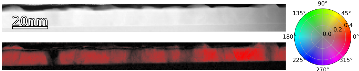
Figure S4: Upper: HAADF image of the large area of this film with carbon to the top, film in the middle, and LSAT substrate at the bottom. Lower: large area mapping of the direction of the d -axis for this film of LCMO on LSAT. All colour mapping of directions referenced to the image axes. d consistently lies close to in-plane suggesting that the b axis is in-plane for much of the film.
