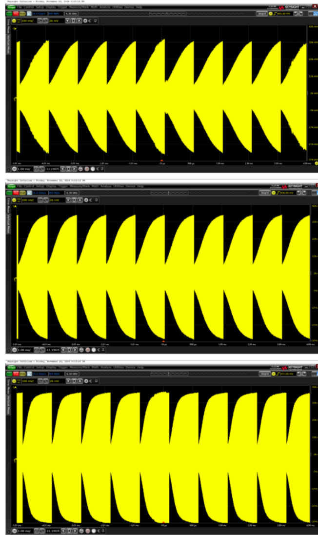
Supplementary Figure 2 The distorted waveforms received by the direct-RF-sampling oscilloscope when the baseband inputs of STD-Metasurface are asymmetric sawtooth waveforms with different high levels. (720mV, 820mV, 1120mV).
