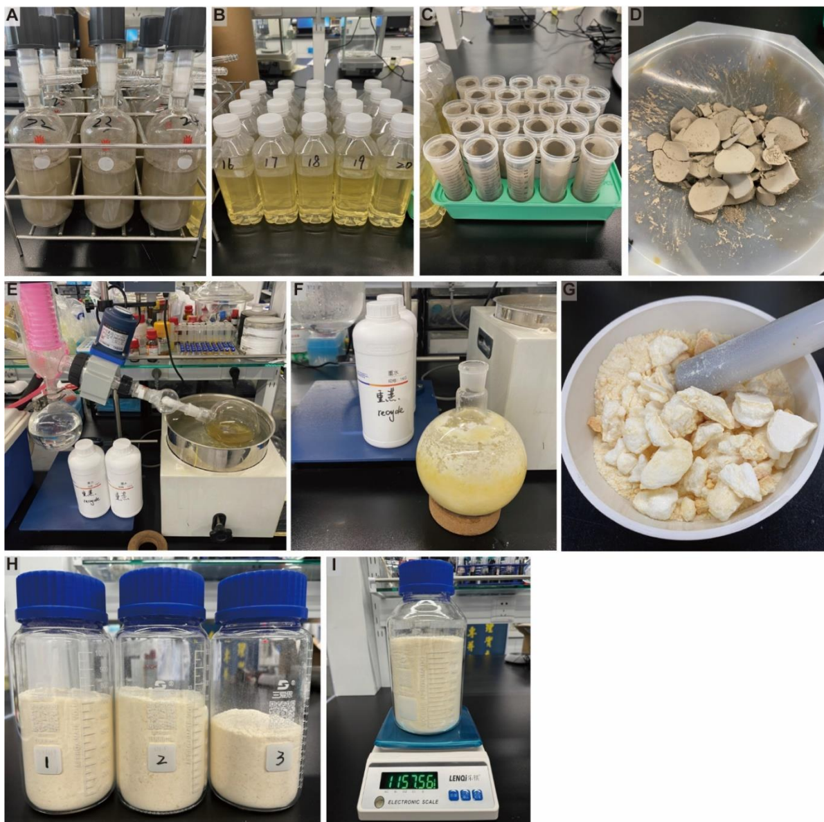
Supplementary Figure 38. Isolation processes of used D 2 O, photocatalysts, and deuterated products. (A) 30 bottles of reaction suspensions after photocatalytic HIE. (B-C) Supernatants and used photocatalysts separated by centrifuging. (D) The powders of used photocatalysts after drying in air at 100 °C for 12 h (they can be employed in the next round of photocatalytic HIE reactions). (E) The rotary evaporation of supernatants in vacuum (the used D 2 O could be obtained). (F) The deuterated products and used D 2 O separated from evaporation. (G) The powders of deuterated products after drying in air at 60 °C for 12 h. (H) The isolated deuterated products from the 1 st , 2 nd and 3 rd round of photocatalytic HIE reactions. (I) The deuterated products in total collected from three rounds of photocatalytic HIE reactions.
