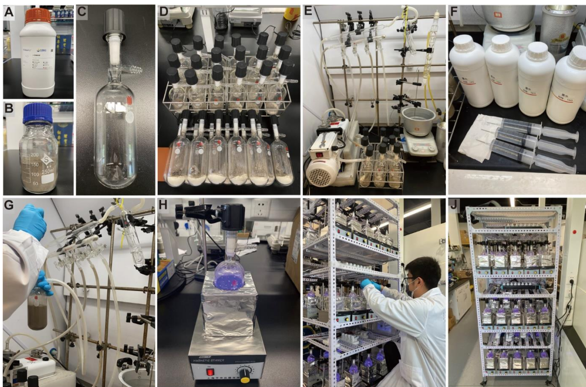
Supplementary Figure 37. The operation process of scale-up photocatalytic HIE reactions. (A) Substrate of 2-aminopyrimidine. (B) 120 g photocatalysts (2.0 wt.% Pd 1 /TiO 2 -h). (C) 250 mL Schlenk bottle. (D) 30 Schlenk bottles (250 mL for each bottle) filled with substrates and photocatalysts. (E) Purging with the Schlenk Line in Ar atmosphere for 3 times. (F) 4.5 L D 2 O. (G) Adding D 2 O. (H) 250 mL batch-mode photoreactor equipped with 410 nm LED strips covered by Al foils. (I) Loading photoreactors. (J) Photoreactor bed equipped with 30 photoreactors in operation.
