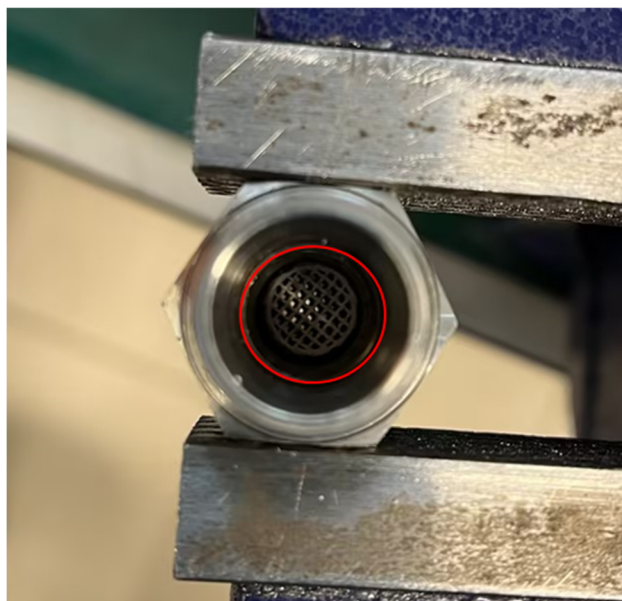
Fig. S42 Custom-sizing of 3D-printed catalysts to fit specific reactor dimensions.
