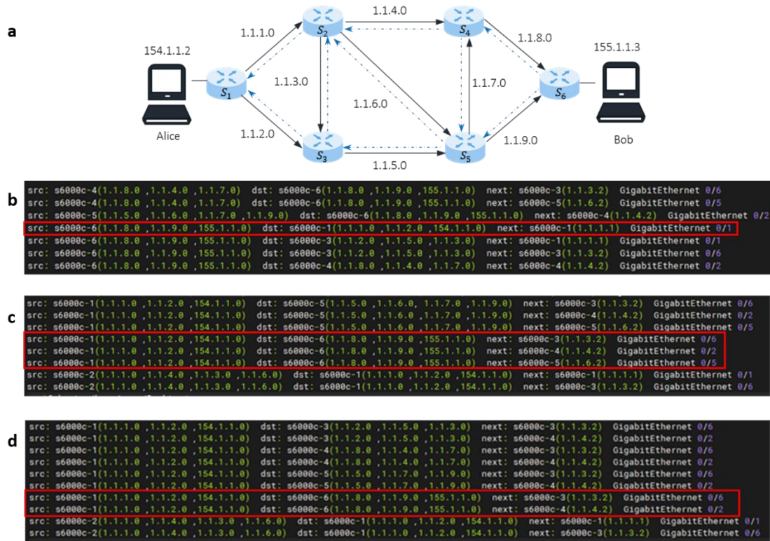
SUPPLEMENTARY FIG. 1. An implementation of the multipath search algorithm. a , A real transmission network with 6 NC-integrated layer-3 switches. All the nodes and the solid directed lines connecting them consist of a directed acyclic graph exactly between router S_1 and S_6 . (b to d) show the routing entries generated at node S_2 under different circumstances. b , Only one next hop to the router S_1 . c , Three next hops to the router S_6 . d , Two next hops remain to the destination. Dynamic routing is well supported in the algorithm.
