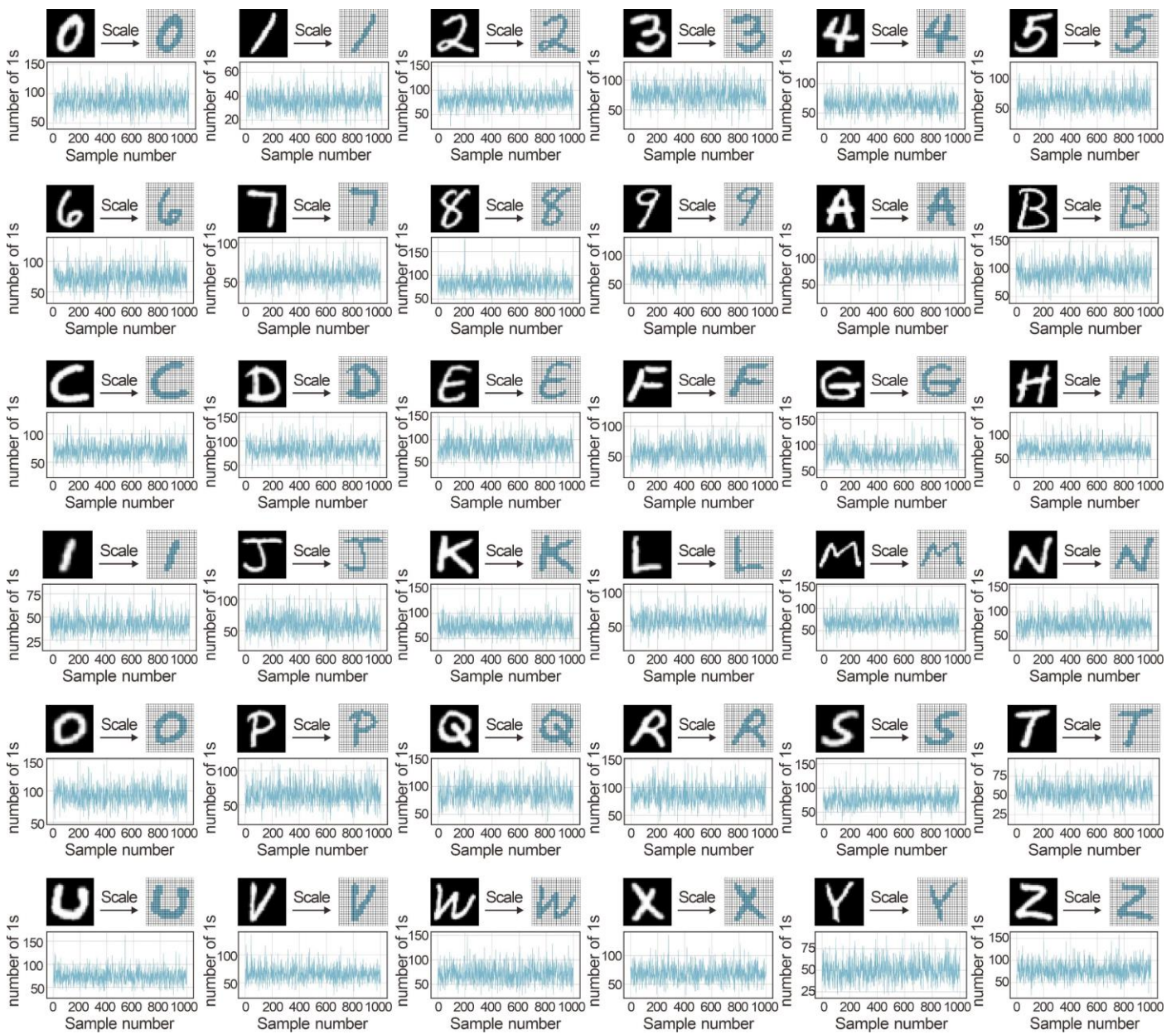
Fig. S23| Determination of 36 input patterns. Top row: All original symbols were rescaled to a 20 \times 20 grid and binarized into 400-bit patterns, with each pixel assigned a value of 1 when exceeding a threshold. Bottom row: The number of 1s in each input pattern.
