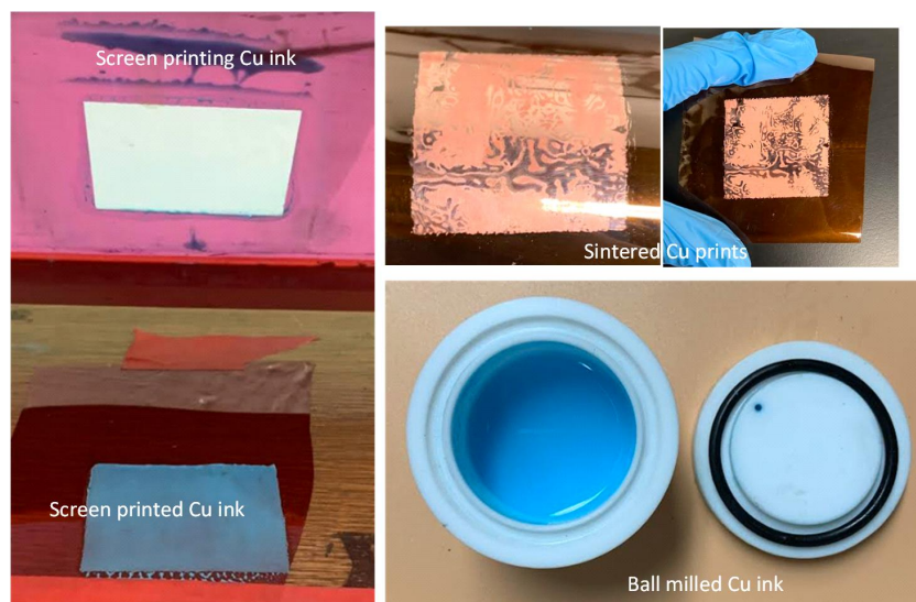
Supplementary Fig. 13 Proposed copper molecular decomposition inks at different stages of preparation: Screen-Printed ink verifying its viscosity and printability, Sintered and ball-milled ink.
