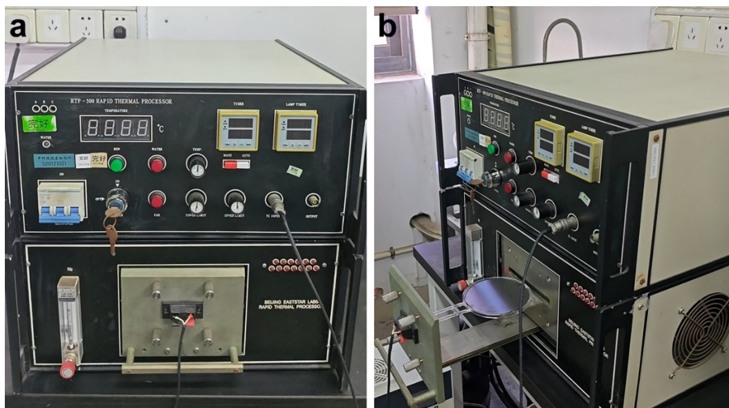
Supplementary Fig. 1 Digital photographs of the (a) RTA device, and (b) quartz holder and silicon wafers inside the device.
