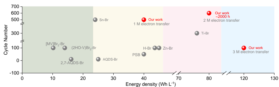
Supplementary Fig. 2. Comparison diagram of cycle number and energy density of different bromine-based flow battery systems. Compared with other bromine-based batteries, the battery system we designed demonstrated absolute advantages in terms of cycle stability and energy density due to the two-electron transfer mechanism and Br 2 -free environment. (See Methods for references for all comparisons).
